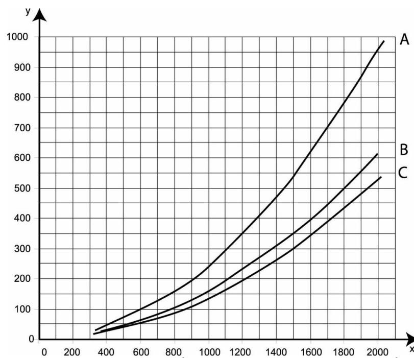
X-axis: m<sup>3</sup>/h Y-axis: Static Pa A: Extension arm bent 40° (to its limit). B: Extension arm bent 90°. C Extension arm is straight.
